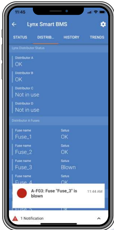
Lynx Smart BMS alarms on the VictronConnect App and a GX device
